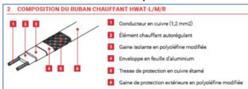
Figure 8 - Composition du Ruban HWAT
