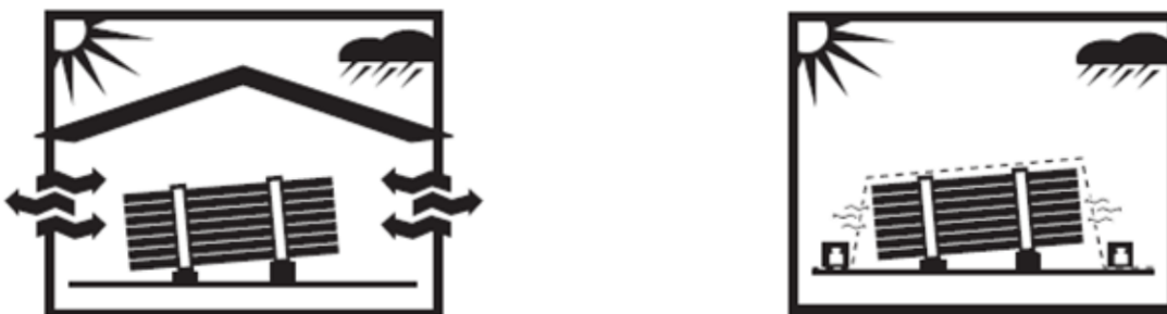
Figure 28 – Stockage des bacs Kalzip®
