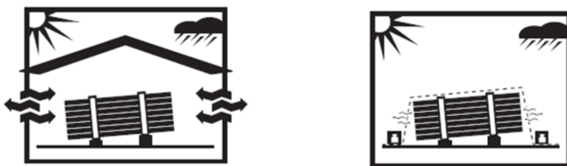
Figure 19 – Stockage des bacs Kalzip®
