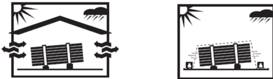
Figure 22 – Stockage des bacs Kalzip®
