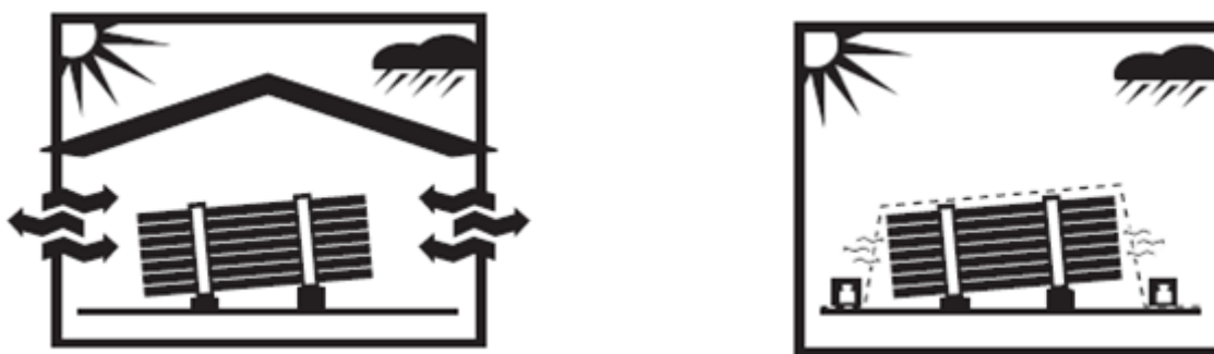
Figure 18 – Stockage des bacs Kalzip®
