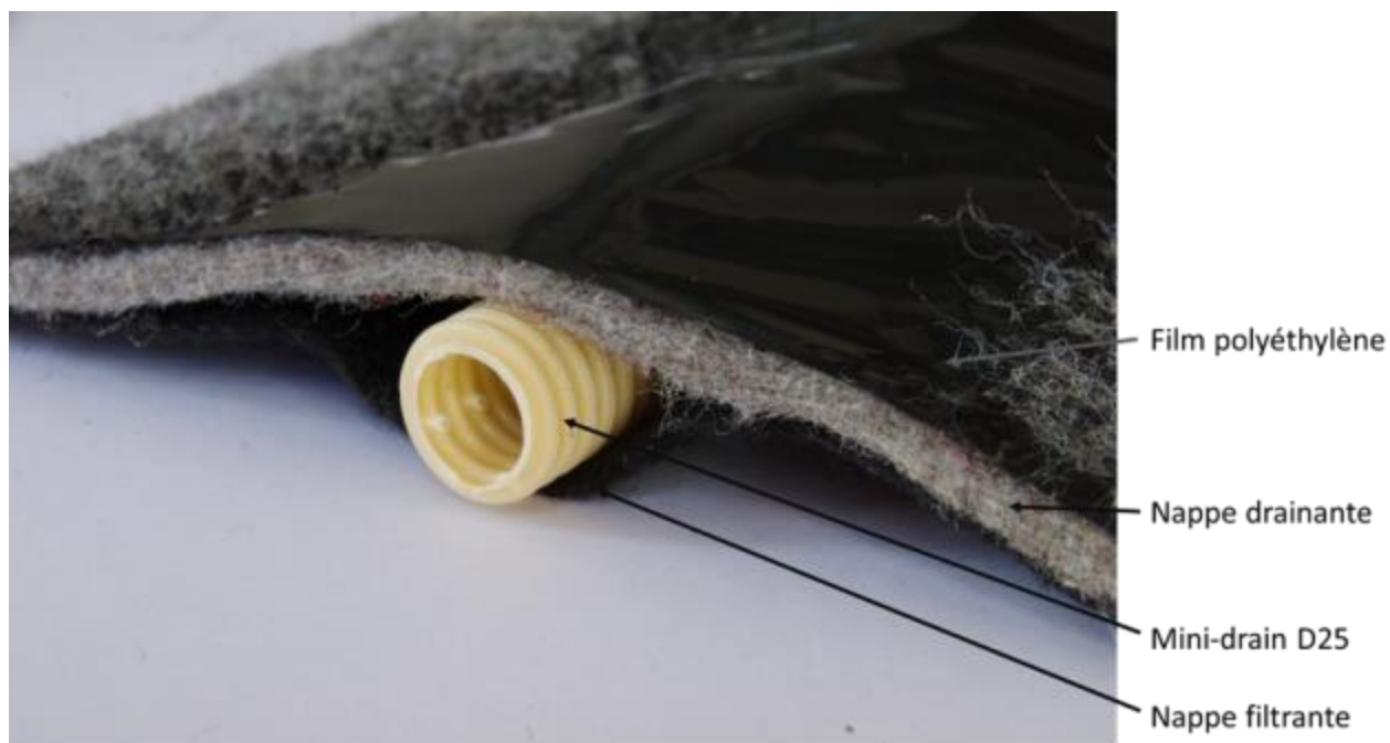
Figure 1 - Composition du DRAINTUBE® FTB
