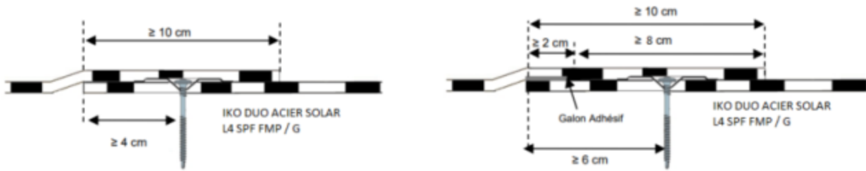
Figure 5 – Recouvrements longitudinaux
